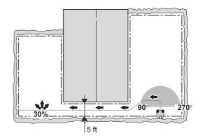
Area: 1.4 acre (5500 m²). Rectangular garden with the charging station placed by an island. A large part of the boundary wire is routed on a slope that is steeper than 10 %. Guide wire recommended.
