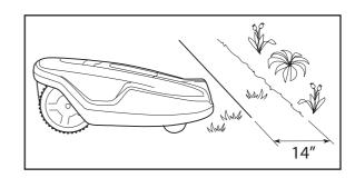
If the working area borders against a flat path or the like that lies level with the lawn, it is possible to allow Automower® to run a little over the path. The boundary wire should then be laid 4" (10 cm) from the edge of the path.
