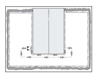
The longer the guide wire, the closer the mower follows the guide wire. If the guide wire is longer than 1000 ft (300 metres), the mower may find it difficult to follow the wire. This varies depending on the design of the garden and installation.
