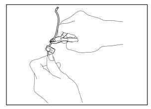
6. Press the connector onto the contact pin, marked A, on the charging station.
