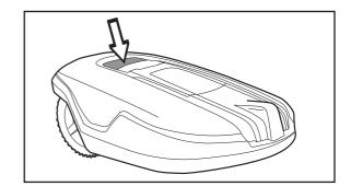
The control panel consists of a display and a keypad. All information is shown on the display and all input is done using the buttons.
