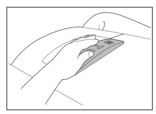
The control panel on the top of Automower® is where you manage all the mower settings. The main switch is also located on the control panel. Open the control panel cover by pressing down the **STOP** button.
