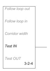
When the function is selected the mower will immediately follow the boundary wire, guide 1 or guide 2, depending on which one it finds first, in to the charging station. If there is a passage and the mower can not run through it, the *Corridor width* value is set too high. When Test IN is activated, the mower runs at the greatest distance from the wire that the selected corridor width permits.
