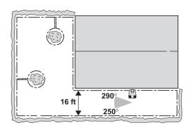
Area: 0.85 acre  $(3500 \text{ m}^2)$ . U-shaped garden with the charging station placed on one of the large open areas. Guide wire recommended through the passage.
