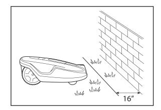
If the working area borders against a small ditch, for example, a flower bed or a small elevation, e.g. a low verge (1" - 2")((3 - 5 cm)), the boundary wire should be laid 14" (35 cm) inside the working area. This prevents the wheels from driving into the ditch or up onto the verge.
