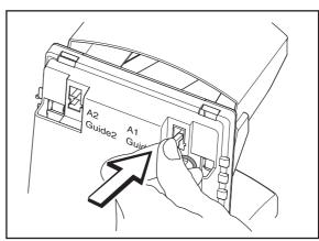
7. Refit the cover on the charging station. Ensure the three guides on the charging station enter the right holes in the cover.
