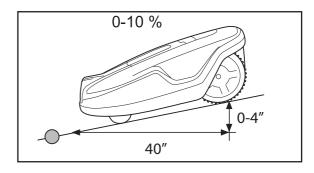
The boundary wire should not be laid across a slope that is steeper than 10 %. There is a risk of Automower® finding it difficult to turn there. The mower will then stop and show the fault message *Outside working area*. The risk is at its greatest in damp weather conditions, as the wheels can slip on the wet grass.
