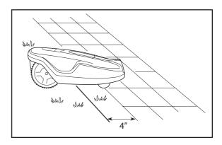
When the working area is divided by a flat slab path that is level with the lawn, it is possible to allow Automower® to run over the path. It can be an advantage to lay the boundary wire under the slabs. The boundary wire can also be laid in the joint between the slabs.
