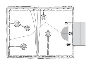
Area: 0.4 acre (1600 m²). L-shaped garden with the charging station placed in the large open area. No guide wire is necessary.
