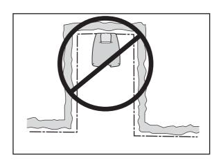
Avoid placing the charging station in a narrow passage (narrower than about 10 ft (3 metres)).
