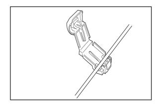
4. Press the connector together using a pair of pliers. Press until you hear a click.
