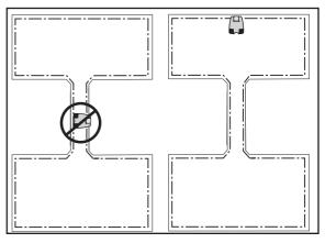
Do not position the charging station so that the mower can come closer than 10 ft (3 metres) behind the charging station (for example on a narrow point). The mower will not then find the charging station.
