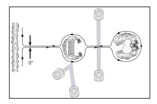
Obstacles that can withstand a collision, for example, trees or bushes higher than 6" (15 cm), do not need to be demarcated by the boundary wire. Automower® will turn when it collides with this type of obstacle.
