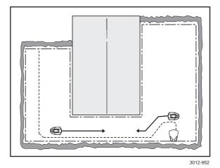
In the passage, the guide wire must therefore be placed so that the robotic lawnmower has as much space to run in as possible. The distance between the boundary loop and the guide wire must however be at least 12"/30 cm.
