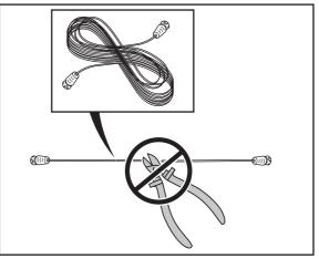
It is possible to let the low voltage cable cross the working area. The low voltage cable must be stapled down or buried, and the cutting height should be such that the blades on the blade disc can never come in contact with the low voltage cable.
