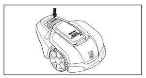
The control panel on the top of the robotic lawnmower is where you manage all the robotic lawnmower settings. Open the control panel cover by pressing down the **STOP** button.
