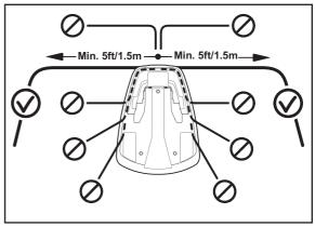
The charging station must be positioned with a great deal of free space in front of it (at least 10ft/3 metres). It should also be centrally placed in the working area to make it easier for the robotic lawnmower to reach all areas in the working area.
