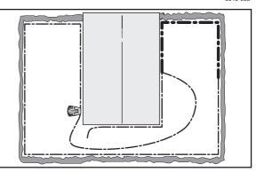
5. When the break is found, the damaged section must be replaced with a new wire. The damaged section can be cut out if it is possible to shorten the boundary wire. Always use original couplers.
