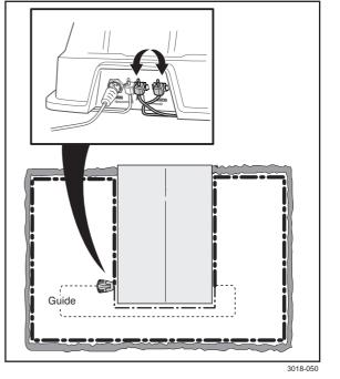
b) Put AL and Guide back in their original positions. Then switch AR and Guide. If the indicator lamp flashes yellow, then the break is somewhere on the boundary wire between AR and the point where the guide wire is connected to the boundary wire (thick black line in the illustration).
