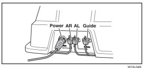
3. Connect the charging station to the power supply. Switch the connections between the guide wire and the boundary wire in the charging station.
