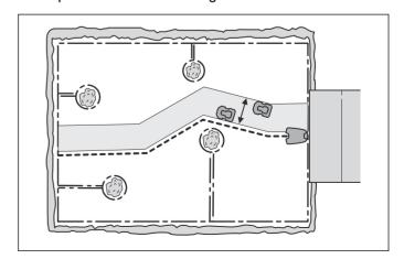
The robotic lawnmower runs at varying distances from the guide wire to reduce the risk of tracks forming. The area beside the wire which the robotic lawnmower then uses is called the Corridor.
