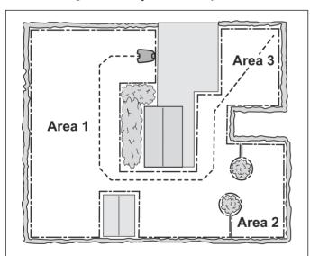
A number of unique selections are required to allow the robotic lawnmower to reach the remote area.
