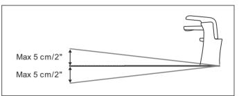
The charging station must not be positioned in a way that can bend its base plate.
