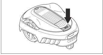
2. Press the **ON/OFF** button and make sure the robotic lawnmower is turned off. Check that the indicator lamp on the **ON/OFF** button is not lit. This means
