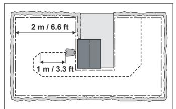
The charging station must be positioned on level ground. The front end of the charging station cannot be positioned higher or lower than the back end according to picture below.
