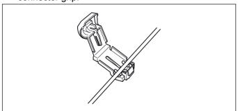
Press the connectors together using a pair of pliers. Press until you hear a click.
