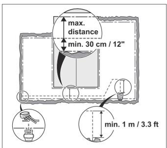
The guide wire, as the boundary wire, can be stapled to or buried in the ground.
