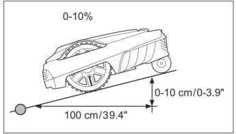
The boundary wire should not be laid across a slope that is steeper than 15%. There is a risk that the robotic lawnmower will find it difficult to turn there. The robotic lawnmower will then stop and the *Outside working area* fault message is displayed. The risk is at its greatest in damp weather conditions, as the wheels can slip on the wet grass.
