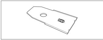
The blades must be in good condition to obtain the best mowing result. In order to keep the blades sharp for as long as possible it is important to keep the lawn free from branches, small stones and other objects.
