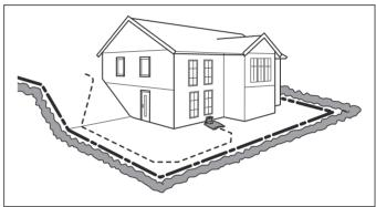
Avoid laying the wire at sharp angles. This can make it difficult for the robotic lawnmower to follow the guide wire.
