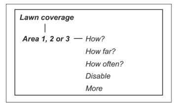
The factory settings allow the robotic lawnmower to follow the guide wire 99 m in 20% of the times it leaves the charging station. If the guide wire in reality is less than 99 m the robotic lawnmower will follow it to the point where the guide wire is connected to the boundary wire.
