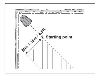
2. When the guide calibration is completed, the robotic lawnmower follows the guide wire and then starts mowing.
