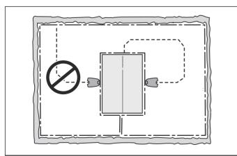
**Note:** Correct placement of the charging station and the guide wire is important for the docking ability of the robotic lawnmower. Read more in *Laying the boundary*
