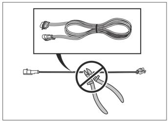
It is possible to let the low voltage cable cross the working area if it is stapled down or buried. The cutting height should be such that the blades can never come in contact with the low voltage cable.
