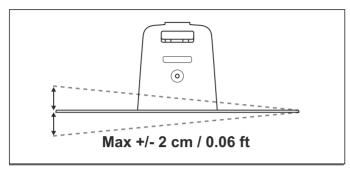
**Note:** Position the charging station on level ground so that the robotic lawnmower has optimal conditions for docking. It is essential that the charging plate is neither bent nor tilted in any direction.
