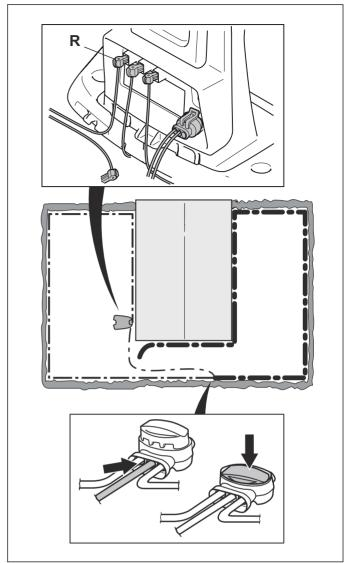
If the indicator lamp now is green, then the break is somewhere in the wire between the disconnected end to the point where the new wire is connected (thick black line below). In that case, move the connection for the new wire closer to the disconnected end (roughly at the middle of the suspected wire section) and check again if the indicator lamp is green.
