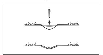
The low voltage cable must never be stored in a coil or under the charging station's base plate as this can interfere with the signals from the charging station.
