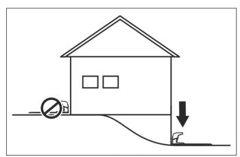
The charging station should not be placed on an island as this limits the laying of the guide wire in an optimal way. If the charging station has to be installed on an island, the guide wire also has to be connected to the island. Read more about islands in the *Boundaries within the working area on page 15*.
