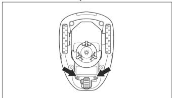
Release the latch of the connector and pull it upwards.
