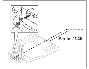
If the guide wire has to be installed on a slope, it is an advantage to lay the wire at an angle to the slope. This makes it easier for the robotic lawnmower to follow the guide wire on the slope.
