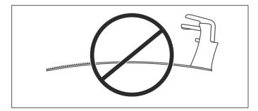
It is also important that the charging station is not bent sideways. Otherwise the robotic lawnmower might have difficulties docking.
