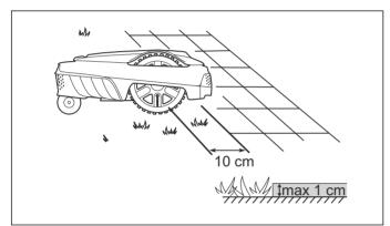
When the working area is divided by a paving stone path that is level with the lawn, it is possible to allow the robotic lawnmower to run over the path. It can be an advantage to lay the boundary wire under the paving stones. The boundary wire can also be laid in the joint between the paving stones. Ensure that the tiles are in level with the lawn to avoid excessive wear on the robotic lawnmower.
