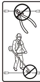
The low voltage cable must not be shortened, extended or spliced.
