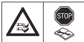
**WARNING:** Operate the disabling device before working on or lifting the machine.
