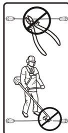
The low voltage cable must not be shortened, extended or spliced.
