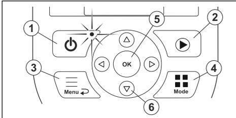
1. The **ON/OFF** button is used to turn the product **ON/OFF**. The indicator lamp on the **ON/OFF** button is an important status indicator. Refer to *The indicator lamp on page 29*.
