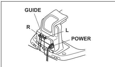
3. Switch the connections between the guide wire and the boundary wire in the charging station.
