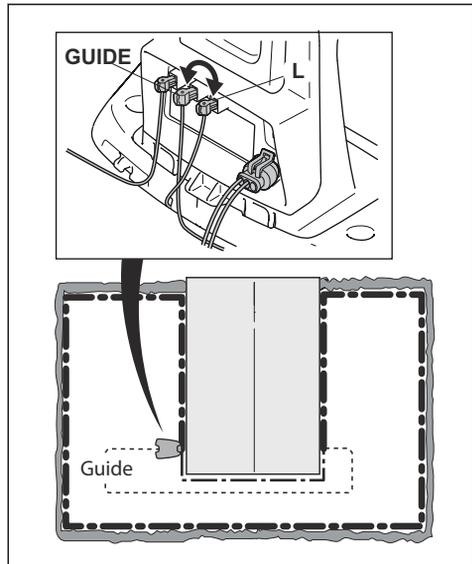
To rectify the fault you will need boundary wire, connector(s) and coupler(s):
