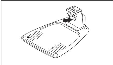
2. Check that the boundary wire connections to the charging station are properly connected and not damaged. Check that the indicator lamp in the charging station is still flashing blue.
