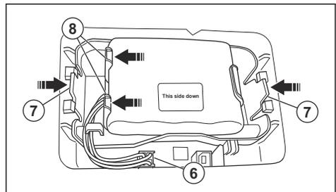
8. Release the latch of the battery and lift up the battery from the battery holder.
