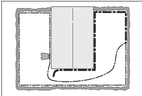
Continue until only a very short section of the wire remains which is the difference between a solid green light and a flashing blue light. Then follow instruction in step 5 below.
