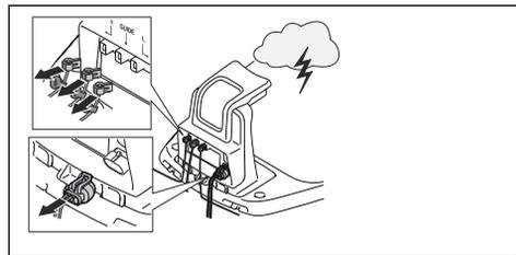
To reduce the risk of damage to electrical components in the product and the charging station, we recommend that all connections to the charging station are disconnected (power supply, boundary wire and guide wire) if there is a risk of a thunderstorm.
