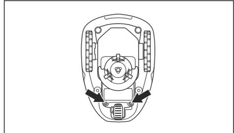
6. Release the latch of the connector and pull it upwards.
