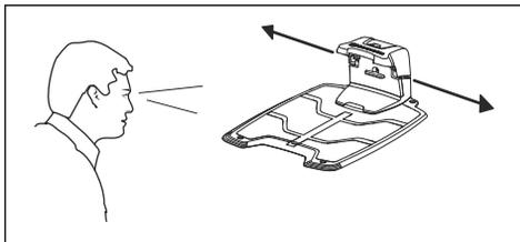
If the distance on the left side of the starting point is less than 0.6 m / 2 ft. the calibration process is interrupted. For the widest possible guide corridor, make sure that the distance from the starting point to the boundary wire is minimum 1.35 m / 4.5 ft. (perpendicular to the guide wire).
