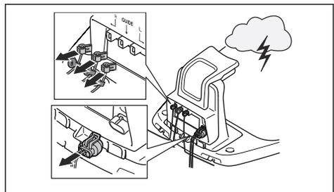
To reduce the risk of damage to electrical components in the product and the charging station, we recommend that all connections to the charging station are disconnected (power supply, boundary wire and guide wire) if there is a risk of a thunderstorm.
