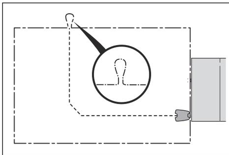
**Note:** Make a blueprint of the work area before you install the boundary wire and guide wire.
