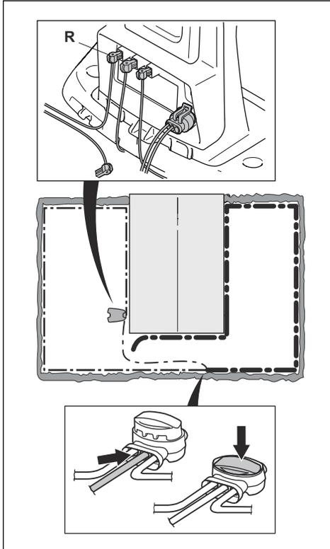
If the indicator lamp now is flashing yellow, then the break is somewhere in the wire between the disconnected end to the point where the new wire is connected (thick black line below). In that case, move the connection for the new wire closer to the disconnected end (roughly at the middle of the suspected wire section) and check again if the indicator lamp is green.
