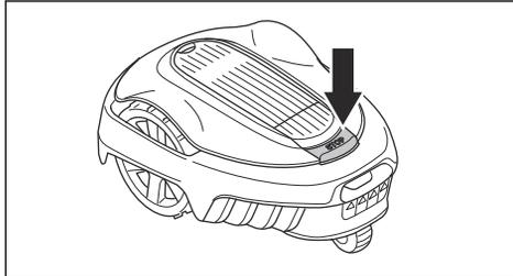
2. Push the **ON/OFF** button for 3 seconds and make sure the product is switched off. Check that the indicator lamp on the keypad is not lit. This means that the product is disabled. Refer to *Indicator lamp in the charging station on page 48*.
