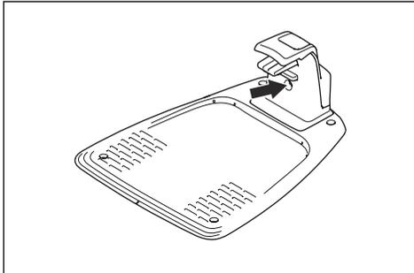
2. Check that the boundary wire connections to the charging station are properly connected and not damaged. Check that the indicator lamp in the charging station is still flashing blue.
