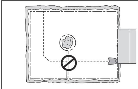
To make an island, isolate areas in the work area with the boundary wire. We recommend to isolate all stable objects in the work area.
