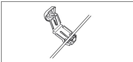
3. Close the connector with a pair of pliers.
