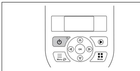
4. Check that the indicator lamp on the keypad is not lit.
