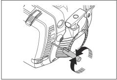
b) Turn the idle speed screw T counterclockwise until the cutting attachment stops.
