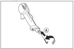
If the start throttle speed is more than 6500 rpm, turn the adjuster screw (A) counterclockwise. When the cutting attachment starts to rotate, turn the adjuster screw (A) 1/2 turn.
