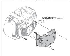
Replace the air paper filter with a nylon air filter that is approved for operation in winter conditions. Refer to, To change from a paper air filter to a nylon air filter on page 25.
