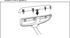
2. Put the guard extension into position on the cutting attachment guard with the 4 locking hooks.
