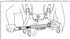
12. Adjust the height of the suspension point. Refer to Product overview on page 2. For forestry clearing, the correct height of the suspension is approximately 10 cm/4 in below your hip.
