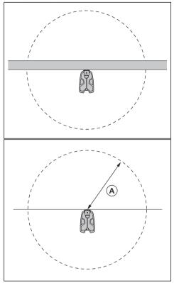
**Note:** The product uses the charging station signal to search for the charging station when it is in the docking area.
