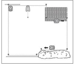
Put the product to straddle the edge between the lawn and the stone path if it is less than 1 cm / 0.4 in. high when you add a waypoint.
