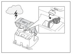
To decrease the risk of damage to electrical components in the product and the charging station, we recommend that the power supplies to the charging station and reference station are disconnected if there is a risk of a thunderstorm. Connect the power supplies again when there is not a risk of thunderstorm.
