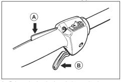
Release the throttle trigger lockout and make sure that the throttle control is locked at idle speed.
