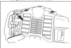
Turn the idle speed screw T counterclockwise until the cutting attachment stops.
