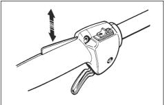
Make sure that the throttle control and throttle trigger lockout move freely and that the return springs operate correctly.
