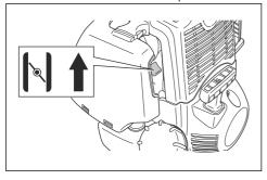
Push the air purge bulb until fuel starts to fill the air purge bulb.
