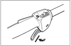
Push the throttle trigger lockout and make sure that it goes back to its initial position when you release it.
