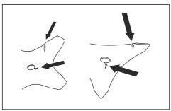
Examine the support flange for cracks. Replace the support flange if it is damaged.
