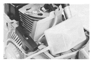
In order to get at the air filter, remove the cylinder cover by undoing the three retaining screws and lifting the cover off upwards—backwards.
