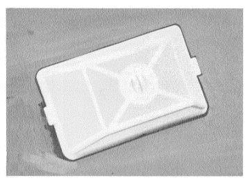
Rinse the filter in warm soap suds. Do not rinse in fuel. Reassemble the filter and make sure that it lies close to the carburettor. Use two filters alternately. Clean the filter daily.
