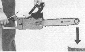
Use the following procedure to check that the automatic chain brake actuates correctly;
