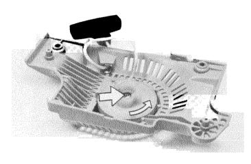
Pull out the cord approx. 30 cm and lift up into the notch in the periphery of the pulley. Zero-set the return spring by letting the pulley rotate slowly backwards. Undo the screw in the centre of the pulley. If necessary, remove the return spring and change it.
