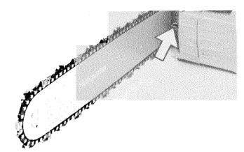
E. Tension the chain while holding up the bar tip. Do not tension the chain stronger than it can be pulled around by hand.
