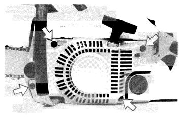
Loosen the four screws that retain the starter. Remove the starter.
