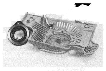
Lubricate the new spring with engine oil.
