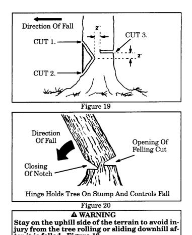
ter it is felled. Figure 18. <u>NOTE:</u> Before the felling cut is complete, use wedges to open the cut when necessary to control the direction of fall. Use wood or plastic wedges, but *never* steel or iron, to avoid kickback and chain
