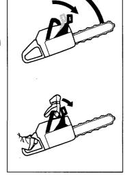
7 During felling your left hand grasps the front handle in such a way that it cannot activate the safety trigger. In this position the chain brake can only be activated by the inertia action of the counterweight.
