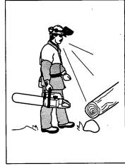
Take the utmost care when cutting through branches or logs that are in tension. A log or branch that is in tension can suddenly spring back into its natural position before or after you cut it. If you stand on the wrong side or start cutting in the wrong place it may strike you or your chain saw. This could make you lose control and cause a serious accident.
