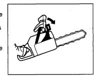
3 You can also use the chain brake as a temporary brake when you change position or if you put the saw down for a short time. You should also apply the chain brake manually if there is a risk of the chain accidentally hitting anyone or anything close by.
