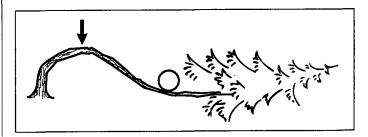
b) Decide which is the SAFEST way to release the tension and whether YOU are able to do it safely. In complicated situations the only safe method is to put aside your chain saw and use a winch.
