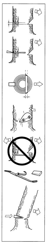
We recommend that you use a bar that is longer than the diameter of the tree, so that you can make the FELLING CUT and DIRECTIONAL CUT with single cutting stokes. (See "Technical data" to find out which lengths of bar are recommended for your saw).
