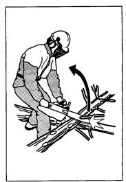
4 Never use the saw above shoulder height and try not to cut with the tip of the bar.
