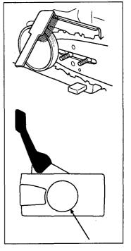
Regularly check that the brake band is at least 0.6 mm thick at its thinnest point.
