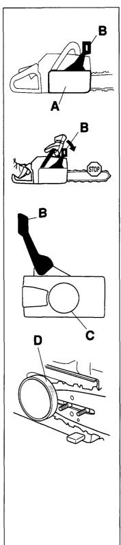
2 The safety trigger is designed solely to activate the chain brake. Another important safety feature is that it prevents the chain from hitting your left hand if you lose your grip on the front handle.
