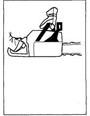
The way the chain brake is triggered, either manually or automatically, depends on the force of the kickback and the position of the chain saw in relation to the object that the kickback zone of the bar strikes.
