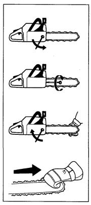
The position of the chain tensioning screw varies from model to model. See the "What is what" section to find out where it is on your saw.
