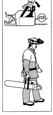
4 To release the chain brake pull the safety trigger backwards, towards the front handle.
