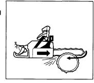
7 Follow the instructions on sharpening and maintaining your bar and chain. When you replace the bar and chain use only combinations that are recommended by us. See the sections on "Cutting equipment" and "Technical dat
