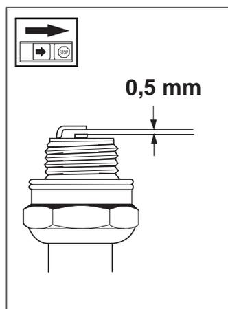
**If the machine is low on power, difficult to start or runs poorly while idling always check the spark plug first before taking any other action.**
