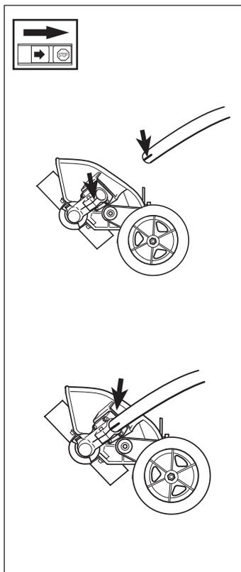
**NOTE!** Do not forget to remove the locking pin before using the machine.
