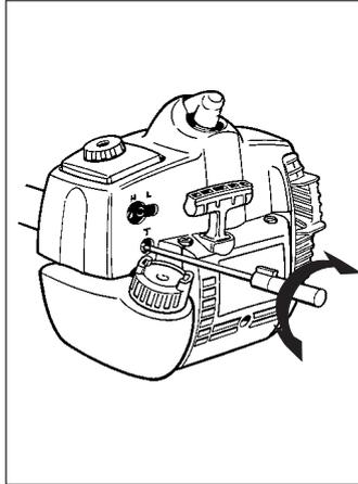
**CAUTION!** Contact your servicing dealer, if the idle speed setting cannot be adjusted so that the cutting attachment stops. Do not use the machine until it has been properly adjusted or repaired.
