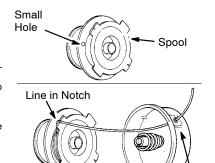
Wind the line evenly and tightly onto the spool. Wind in the direction of the arrow found on the spool.
