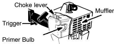
**WARNING:** The trimmer head will turn while starting the engine. Avoid any contact with the muffler. A hot muffler can cause serious burns.
