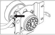
4. Using a brake spoon, turn the brake adjuster towards the front of the unit until the brake begins to engage. The adjuster should then be backed off three clicks.
