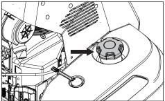
Read the safety instructions before refueling. The capacity for the tank is 6-1/2 gallons (24.6 liters). Regularly check the gas cap gasket for damage and keep the cap properly tightened.
