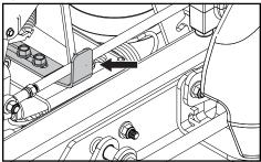
The hydraulic release allows the mower to be moved by hand when not running. See *Moving Machine By Hand* in the *Maintenance* section.
