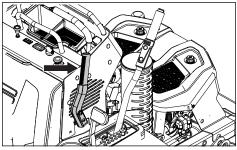
The park brake is found on the right side of the control console. Pull the lever back to engage the brake and push forward to release it.
