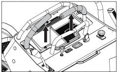
The machine's direction is variable using the two steering controls. The steering controls can be moved forward and back from a neutral position. See **Steering** in the *Operation* section.
