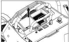
Located in front of the steering controls, the speed control bar is used to change ground speeds. Move the steering controls closer to (for faster speed) or away from (for slower speed) the speed control bar.
