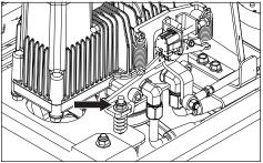
Tighten the nut to bias the unit toward reverse and loosen the nut to bias it forward. During adjustment of the nut, bump the controls into forward and/or reverse and let the controls snap back to neutral. When the wheel is stationary at the same time as the operator controls are in a neutral, tighten the socket cap screws to  $75 \pm 15$  ft-lbs. If the wheel continues to move, further adjustment is required.
