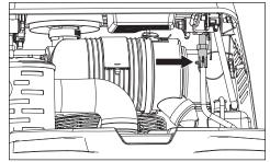
Adjust the nylon coupler until the desired speed is achieved. When the unit tracks straight and is at appropriate maximum forward speed, reinsert the retaining clip to lock the coupler in place.
