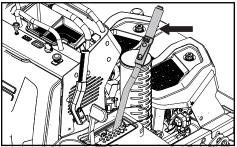
To set the deck cutting height, press the button on the top of the height pin to remove it. Slip the height pin into the hole for the desired cutting height.
