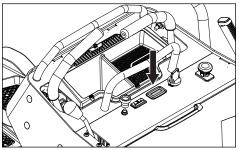
The service meter is located on the left hand control panel and shows the total operating time with the blades engaged.
