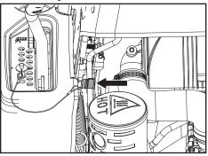
The valve is off when the handle tab is turned perpendicular to the fuel line.
