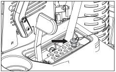
The cutting height can be set from 1-1/2"- 5" (38 mm - 127 mm).
