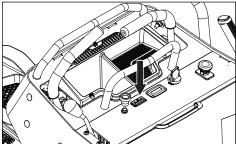
Fuel gauge for the fuel tank is located on the control panel. Sensors will indicate fuel levels. The meter will flash yellow when the tank levels approximately one gallon (3.8 liters).
