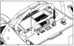
The ignition switch is used to start and stop the engine.
