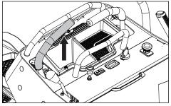
The left steering control is also the Operator Presence Control (OPC). The lever must be down and parallel with the right lever for operation.
