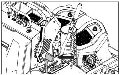
The transport latch will set the deck to the transport height of 5" when the lift lever is pulled back. The latch can also used to mow at the 5" cutting height.
