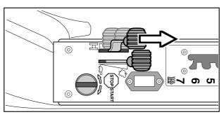
7. Set the required engine speed with the throttle control.
