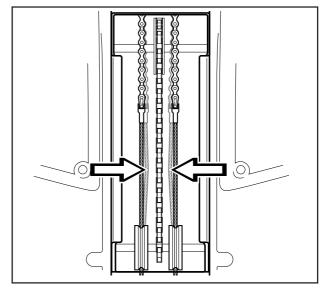
3. When necessary the wires can be tensioned by tightening the adjusting nuts (one on each side of the machine).
