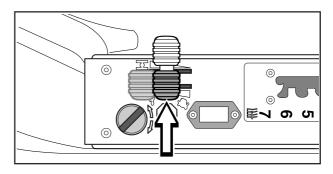
3. If the engine is cold move the choke lever backwards to its end position.
