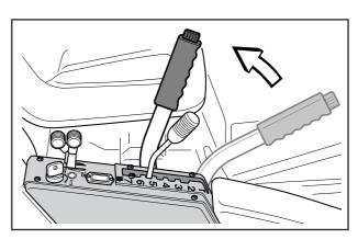
Lifting of the cutting unit
