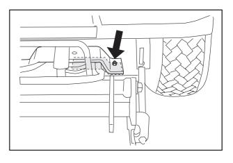
4. Hook on the spring for the blade brake.
