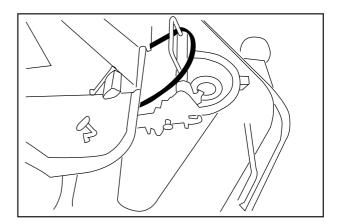
9. Loosen the height setting arm by moving the rear section upwards. When dismantling the cutting unit, off-load the arm by pulling the frame's front section upwards.
