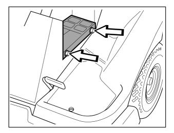
Check the tension of the steering wires by pushing them together (at the arrows). It should be possible to push them together so that the distance between them is half as much, without using unnecessary force.
