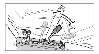
4. Push in the lock button on the lift lever and lower down the cutting unit.
