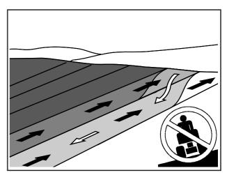
Cut slopes upwards and downwards, not sideways.
