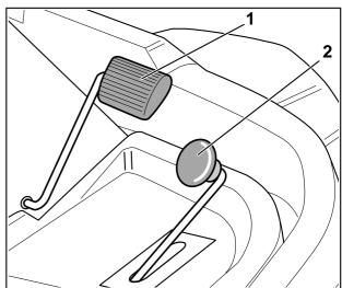
3. Select the required cutting height (1–7) with the cutting height lever.
