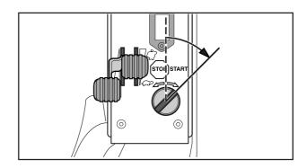
5. When the engine starts release the ignition key immediately back to neutral position.
