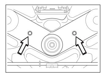
3. Loosen the nuts on the eccentric plate and turn this away.
