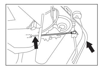
10. Pull the handle and unit simultaneously. Release the handle when the unit has come out a little.
