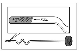
The oil is filled in the same hole as the dip stick.
