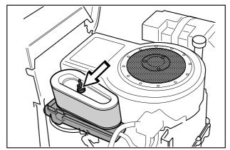
4. Pull off the foam plastic pre-filter from the paper filter and wash clean in mild detergent.
