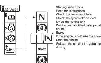
Starting instructions Read the instructions Check the engine's oil level Check the hydrostat's oil level Lift up the cutting unit Put the gear shift/hydrostat pedal in neutral Brake If the engine is cold use the choke
