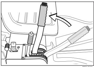
*Lifting of the cutting unit (transport position)*
