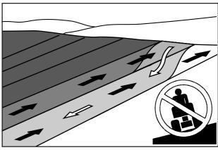
Mow upwards and downwards on slopes, not sideways.
