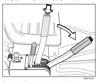
Lowering of the cutting unit (cutting position)
