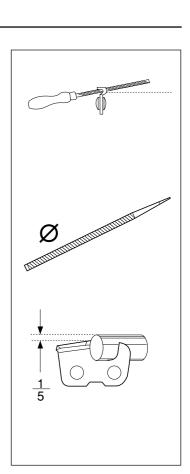
It is very difficult to sharpen a chain correctly without the right equipment. We recommend you to use a file gauge. This will help you obtain the maximum kickback reduction and cutting performance from your chain.
