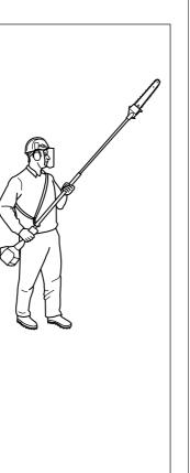
Observe great care when working close to overhead power lines. Falling branches can result in short-circuiting.
