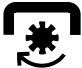
ATTACHMENT CLUTCH ENGAGED
