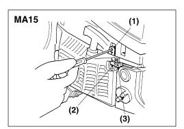
4. Make a test cut adjust the H needle for best cutting power, not for maximum speed.
