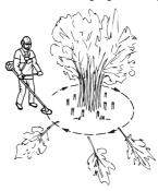
Avoid cutting with the area of the blade between the 12 o'clock and 3 o'clock positions.
