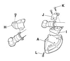
Remove the mounting plate (H). Fit the adapter (I) and bracket (J) with the two screws (K) as shown. Fit the blade guard (A) to the adapter using the 4 screws (L) as shown.
