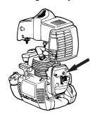
Some mufflers are equipped with a special spark arrestor mesh. If your machine has this type of muffler, you should clean the mesh at least once a week. This is best done with a wire brush. On mufflers without a catalytic converter the mesh should be cleaned weekly, or replaced if necessary. On mufflers fitted with a catalytic converter the mesh should be checked, and if necessary cleaned, monthly. If the mesh is damaged it should be replaced.
