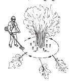
Avoid cutting with the area of the blade between the 12 o'clock and 3 o'clock positions.
