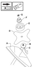
Hook the blade guard/combination guard (A) onto the fitting on the shaft and secure with the bolt.
