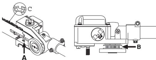
Tension the chain by turning the chain tensioning screw clockwise using the combination spanner. The chain should be tensioned until it does not sag from the underside of the bar.
