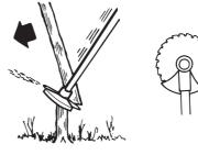
To fell to the right, the bottom of the tree should be pushed to the left. Tilt the blade and bring it diagonally up to the right. Cut with the area of the blade between 3 o'clock and 5 o'clock so that the direction of rotation of the blade pushes the bottom of the tree to the left.
