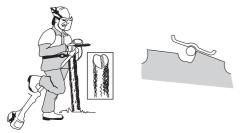
The filing angle is 15°. File alternate teeth to the right and those in between to the left. If the blade has been heavily pitted by stones it may be necessary to dress the top edges of the teeth with a flat file, in exceptional cases. If so, this should be done before filing with a round file. The top edges must be filed down by the same amount for all the teeth.
