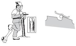
The filing angle is 15°. File alternate teeth to the right and those in between to the left. If the blade has been heavily pitted by stones it may be necessary to dress the top edges of the teeth with a flat file, in exceptional cases. If so, this should be done before filing with a round file. The top edges must be filed down by the same amount for all the teeth.
