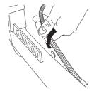
• Put on the harness and hang the machine from the support hook. Now make a final adjustment so that the machine is in a comfortable working position when it hangs from the harness. Tighten the knob.
