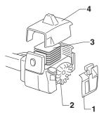
Clean the cooling system with a brush once a week, more often in demanding conditions. A dirty or blocked cooling system results in the machine overheating which causes damage to the piston and cylinder.
