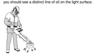
If the chain lubrication is not working:
