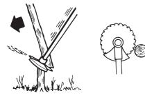
To fell to the right, the bottom of the tree should be pushed
