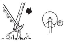
To fell a tree forwards, the bottom of the tree should be pulled backwards. Pull the blade backwards with a quick, firm movement.
