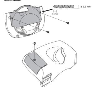
These reduce the cooling air and prevent large amounts of snow from being sucked into the engine.
