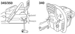
The chain is correctly tensioned when it does not sag from the underside of the bar, but can still be turned easily by hand. Hold up the bar tip and tighten the bar nuts with the combination spanner.
