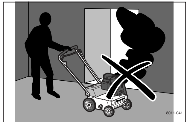
The engine exhaust is poisonous. Never run the engine indoors.
