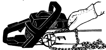
Place chain onto the sprocket
