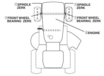
①GENERAL PURPOSE GREASE ②REFER TO MAINTENANCE "ENGINE" SECTION
