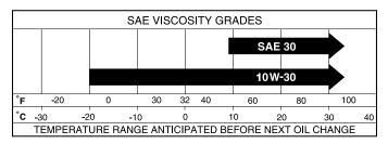
**NOTE:** Multi-viscosity oils (5W30, 10W30 etc.) improve starting in cold weather, and you should check your engine oil level frequently to avoid possible engine damage from running low on oil.
