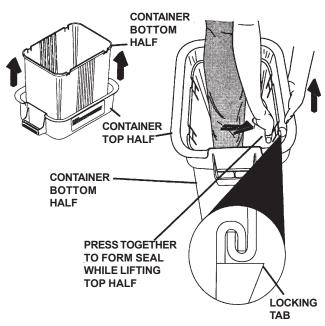
**ASSEMBLY CHECK:** Squeeze sides of lower half of container and check that there is no gap between upper and lower halves. If a gap appears, unlock tabs to separate container halves and repeat instructions above.
