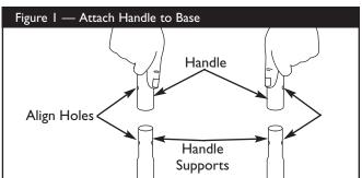
**NOTE:** It may be necessary to move the handle supports from side to side in order to align the handle so it will slide over the handle supports.
