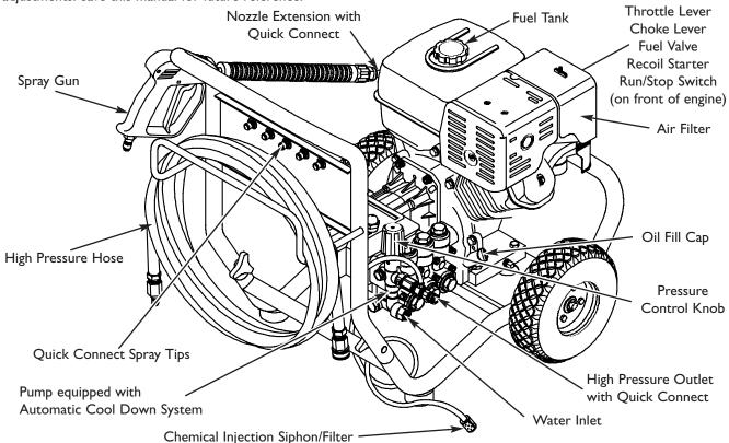
**Air Filter** — Protects engine by filtering dust and debris out of intake air.
