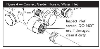
5. Run water through garden hose for 30 seconds to clean out any debris. Turn off water.
