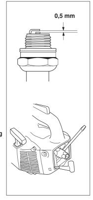
IMPORTANT! Always use the recommended spark plug type. An incorrect spark plug can severely damage the piston/cylinder.
