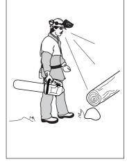
Take the utmost care when cutting through branches or logs that are in tension. A log or branch that is in tension can suddenly spring back into its natural position before or after you cut it. If you stand on the wrong side or start cutting in the wrong place it may strike you or your chain saw. This could make you lose control and cause a serious accident.
