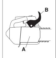
The brake is applied when the front hand guard (B) is pushed forwards.
