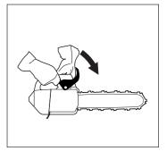
6 The way the chain brake is triggered, either manually or automatically, depends on the force of the kickback and the position of the chain saw in relation to the object that the kickback zone of the bar strikes.
