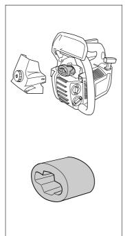
An air filter, which is used for some time, cannot be cleaned completely. Therefore it must be replaced by a new one, with regular intervals.
