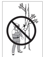
If you have to saw tree limbs or the like that are above shoulder heigth, stand on a work platform or a work stand. Never use the saw while standing on a ladder.
