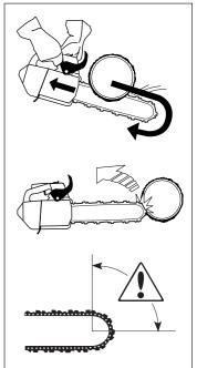
Cutting with the bottom edge of the bar, i.e. from the top of the object downwards, is known as cutting on the pull stroke. In this case the saw pulls itself towards the tree and the front edge of the saw provides a natural rest when cutting. Cutting on the pull stroke gives you better control over the saw and the position of the kickback zone.
