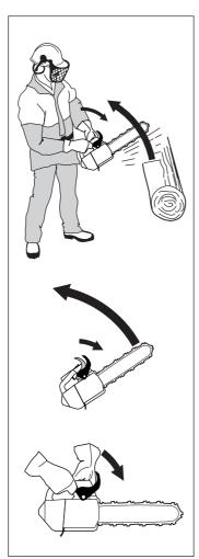
If the kickback is less violent or the kickback zone of the bar is closer to you the chain brake will be activated manually by the movement of your left hand.
