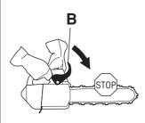
This movement activates a spring-loaded mechanism that tightens the Brake Band (C) around the engine drive system (D) (Clutch Drum).
