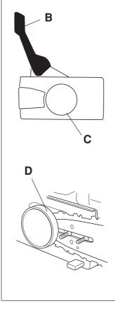
2 The front hand guard is not designed solely to activate the chain brake. Another important safety feature is that it prevents the chain from hitting your left hand if you lose your grip on the front handle.
