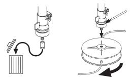
• Screw the trimmer head onto the shaft.
