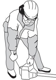
Push the choke control back to its original position as soon as the engine fires, and continue trying to start until the engine starts. When the engine starts, quickly apply full throttle to automatically disengage the start throttle setting.
