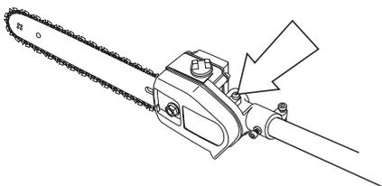
The grease in the bevel gear does not normally need to be changed except if repairs are carried out.
