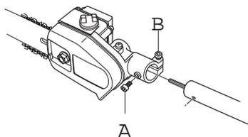
**CAUTION!** Make sure that the drive shaft inside the shaft engages with the cut-out in the cutting head.
