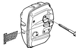
On mufflers without a catalytic converter the mesh should be cleaned weekly, or replaced if necessary. On mufflers fitted with a catalytic converter the mesh should be checked, and if necessary cleaned, monthly. **If the mesh is damaged it should be replaced.**
