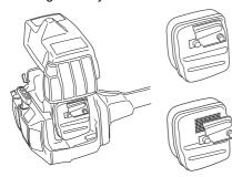
Some mufflers are equipped with a special spark arrestor mesh. If your machine has this type of muffler, you should clean the mesh at least once a week. This is best done with a wire brush.
