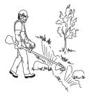
4 Take great care when cutting a tree that is in tension. A tree that is in tension may spring back to its normal position before or after being cut. If you position yourself incorrectly or make the cut in the wrong place the tree may hit you or the machine and cause you to lose control. Both situations can cause serious personal injury.
