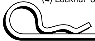
(4) Retainer Springs (double loop)
