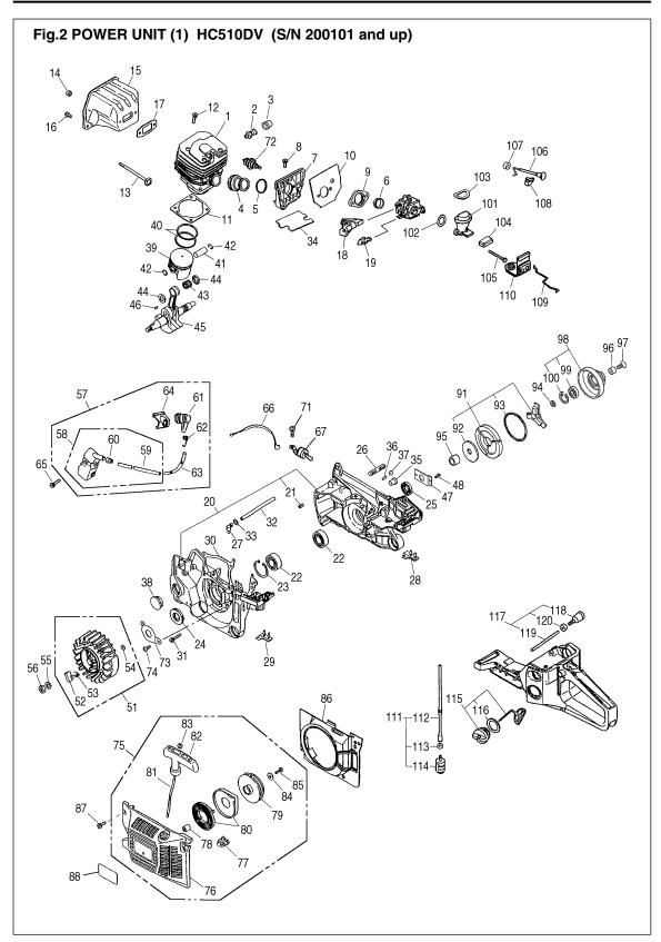
Fig.2 POWER UNIT (1) HC510DV (S/N 200101 and up)
