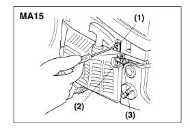
4. Make a test cut adjust the H needle for best cutting power, not for maximum speed.
