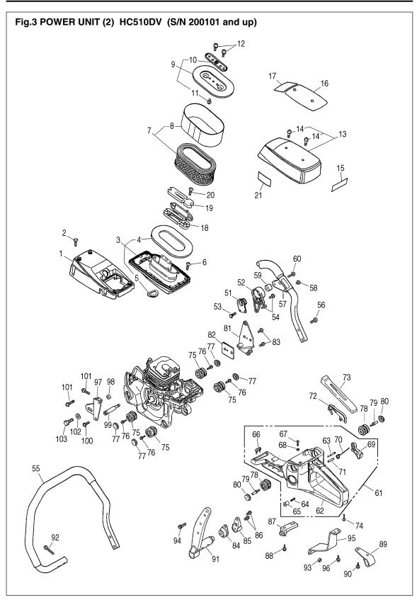
Fig.3 POWER UNIT (2) HC510DV (S/N 200101 and up)
