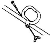
Place handle in comfortable position and tighten securely.
