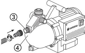
Don't use any hose connection system fittings on the suction side! A vacuum-resistant suction hose must be used
