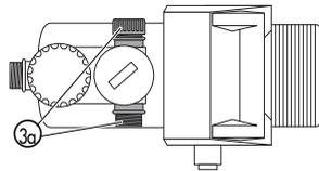
Both pump connectors ③ are equipped with a 33.3 mm (G1) thread to which 13 mm (1/2"), 19 mm (3/4") and 16 mm (5/8") hoses can be connected by using GARDENA hose connection system fittings. The back pump connector is closed with an end cap. Unscrew the end cap for connecting two hoses.
