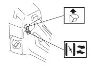
Use the same procedure as for starting a cold engine but without setting the choke control in the choke position. The correct choke/start throttle setting is obtained by moving the choke control to the choke position and then pushing it in again.
