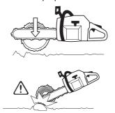
If it is possible (can you turn the log?) stop cutting about 2/3 of the way through the log.
