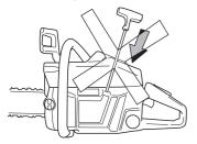
Reactivate the chain brake by pushing the front hand guard back towards the front handle. The chain saw is now ready for use.
