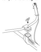
Put on the harness and hang the machine from the support hook. Now make a final adjustment so that the machine is in a comfortable working position when it hangs from the harness.
