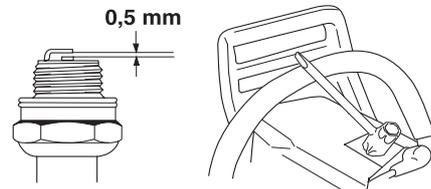
**CAUTION!** Always use the recommended spark plug type! Use of the wrong spark plug can damage the piston/cylinder.
