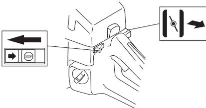
If the machine is fitted with a decompression valve (A): Press the valve to reduce the pressure in the cylinder and make starting easier. You should always use the decompression valve when starting the machine. Once the machine has started the valve will automatically return to its original setting.
