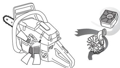
**IMPORTANT!** In order to maintain operation of the centrifugal cleaning system it must be regularly maintained.
