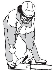
Grip the front handle with your left hand. Hold the chain saw on the ground by placing your right foot through the rear handle. Pull the starter handle with your right hand and pull out the starter cord slowly until you feel a resistance (as the starter pawls engage) then pull firmly and rapidly. **Never twist the starter cord around your hand.**
