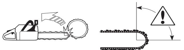
Cutting with the bottom edge of the bar, i.e. from the top of the object downwards, is known as cutting on the pull stroke. In this case the chain saw pulls itself towards the tree and the front edge of the chain saw body rests naturally on the trunk when cutting. Cutting on the pull stroke gives the operator better control over the chain saw and the position of the kickback zone.
