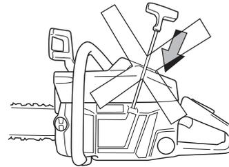
Push in the choke control as soon as the engine fires and keep pulling until the engine starts. When the engine starts, quickly apply full throttle; the throttle start lock will automatically disengage.
