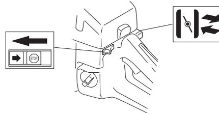
Use the same procedure as for starting a cold engine but without setting the choke control in the choke position. The correct choke/start throttle setting is obtained by moving the choke control to the choke position and then pushing it in again.
