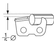
It is very difficult to sharpen a chain correctly without the right equipment. We recommend that you use our file gauge. This will help you obtain the maximum kickback reduction and cutting performance from your chain.
