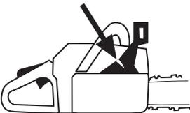
Move the front hand guard forwards and back to make sure it moves freely and that it is securely anchored to the clutch cover.
