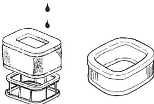
An air filter that has been in use for a long time cannot be cleaned completely. The filter must therefore be replaced with a new one at regular intervals. **A damaged air filter must always be replaced.**
