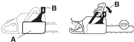
This movement activates a spring-loaded mechanism that tightens the brake band (C) around the engine drive system (D) (clutch drum).
