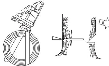
Finish the felling cut parallel with the directional cut line so that the distance between them is at least 1/10 of the trunk diameter. The uncut section of the trunk is called the felling hinge.
