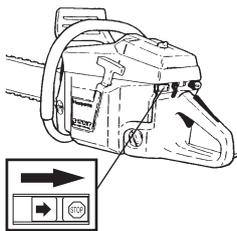
Stop the engine by switching off the ignition. (Move the ignition switch to stop position.)
