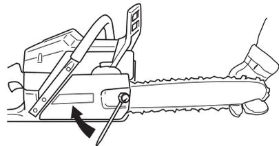
When fitting a new chain, the chain tension has to be checked frequently until the chain is run-in. Check the chain tension regularly. A correctly tensioned chain ensures good cutting performance and long life.
