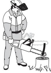
When the bar hits the stump the brake should be applied.
