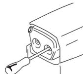
If the muffler on your machine is fitted with a spark arrestor mesh this must be cleaned regularly. A blocked mesh will cause the engine to overheat and may lead to serious damage.
