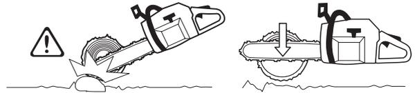
If it is possible (can you turn the log?) stop cutting about 2/3 of the way through the log.
