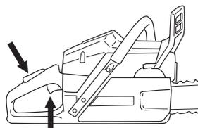
As the chain brake is still engaged the speed of the engine must be set to idling as soon as possible, this is achieved by quickly disengaging the throttle lock. This prevents unnecessary wear to the clutch, clutch drum and brake band.
