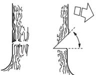
The line where the two cuts meet is called the directional cut line. This line should be perfectly horizontal and at right angles (90°) to the chosen felling direction.
