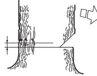
Set the spike bumper (if one is fitted) just behind the felling hinge. Use full throttle and advance the chain/bar slowly into the tree. Make sure the tree does not start to move in the opposite direction to your intended felling direction. Drive a wedge or breaking bar into the cut as soon as it is deep enough.
