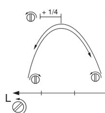
Try to find the highest idle speed by turning the low speed jet L clockwise then anti-clockwise. When the highest speed has been found, turn the low speed jet L 1/4 turn anti-clockwise.
