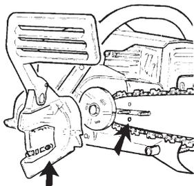
Tension the chain by turning the chain tensioning screw clockwise using the combination spanner. The chain should be tensioned until it does not sag from the underside of the bar.
