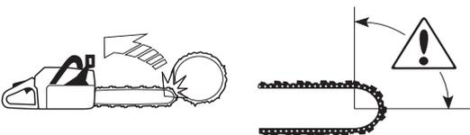
Kickback always occurs in the cutting plane of the bar. Normally the chain saw and bar are thrown backwards and upwards towards the user. However, the chain saw may move in a different direction depending on the way it was being used when the kickback zone of the bar touched the object.
