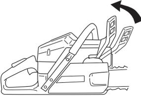
Remove the bar nuts and remove the clutch cover (chain brake). Take off the transportation ring (A).
