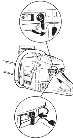
**Note:** It is not necessary to pump continuously. When the extra oil flow has been activated oil consumption increases by 40-80%, depending on the oil pump's basic setting.
