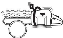
Cutting hardwoods (most broadleaf trees) creates more vibration than cutting softwoods (most conifers). Cutting with cutting equipment that is blunt or faulty (wrong type or badly sharpened) will increase the vibration level. See instructions under the heading Cutting equipment.
