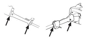
Check that the vibration damping element is undamaged and securely attached.
