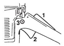
If the machine is fitted with a decompression valve (A): Press the valve to reduce the pressure in the cylinder and make starting easier. You should always use the decompression valve when starting the machine. Once the machine has started the valve will automatically return to its original setting.
