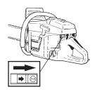
Stop the engine by switching off the ignition. (Move the ignition switch to stop position.)
