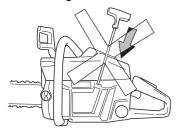
Pull the front hand guard towards the front handle. The chain brake is now disengaged. Your saw is ready for use.
