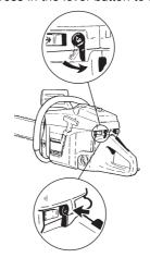
Note: It is not necessary to pump continuously. When the extra oil flow has been activated oil consumption increases by 40-80%, depending on the oil pump's basic setting.
