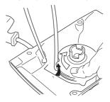
Undo the screw in the centre of the pulley and remove the pulley. Insert and fasten a new starter cord to the pulley. Wind approx. 3 turns of the starter cord onto the pulley. Connect the pulley to the recoil spring so that the end of the spring engages in the pulley. Fit the screw in the centre of the pulley. Insert the starter cord through the hole in the starter housing and the starter handle. Make a secure knot in the end of the starter cord.
